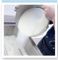
Gelato is produced by continuously stirring a mixture containing milk, sugar and natural flavourings as it freezes. A mixer is an indispensable tool for mixing, homogenising and diffusing any solid or fibrous ingredients into the mix. This helps obtain a consistent, uniform base.
