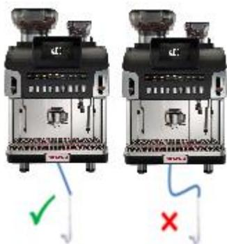
The drain hose must maintain a constant downward slope over the entire length and must not be allowed to kink (see diagram left). Without this, waste coffee grounds can build up and cause blockages requiring a **chargeable** engineer call out.
